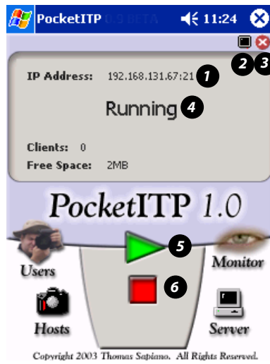
Figure 6.1: Description of the main window controls: (1) The IP Address and socket that the server is running on, (2) The LCD-off button, (3) The exit button, (4) The server status indicator, (5) The start button, (6) The stop button.
