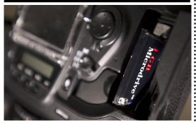
Remove the CF card from your computer and insert it into the camera with the WT-2 attached. Wait for the green light to go out, then press the *Menu* button. Navigate to the *Set Up* tab (wrench icon) and continue on to the next step...
