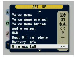
Select the *Wireless LAN* entry and press the controller pad right to configure the WT-2 transmitter.
