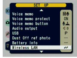
Select the *Wireless LAN* entry and press the controller pad right to configure the WT-2 transmitter.
